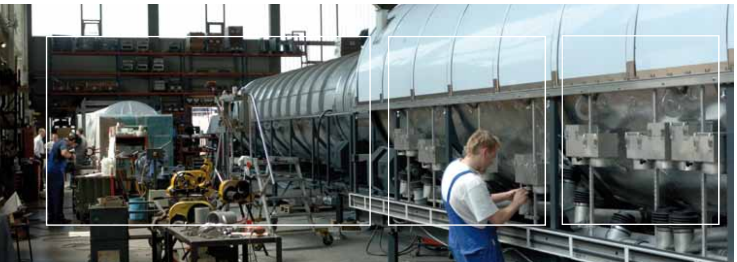
The Lavatec fully automatic Continuous Tunnel Washer, the continuous double drum principle makes the system particularly flexible.
